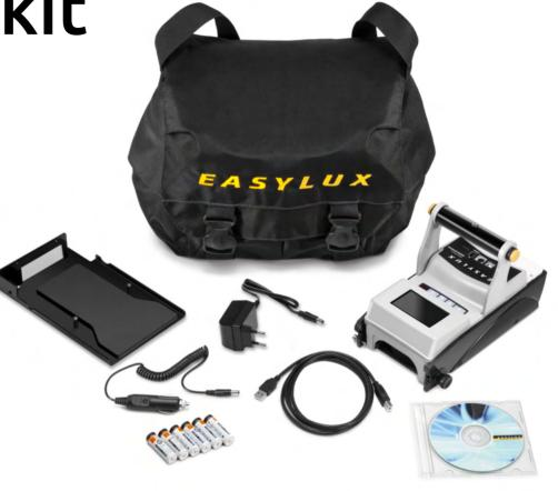
MiniReflecto Horizontal measures the night visibility **RL**, the Day Visibility **Qd**, the visibility under wet **RL** wet and continuous wetting conditions RL-2 rain of all shapes and colors of road markings, even **RL** profiled up to 15 mm without adjustments.
