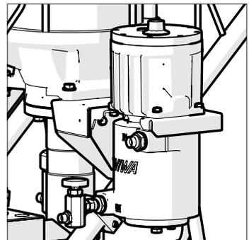
Fig. 12 Material fluid heater on cart
