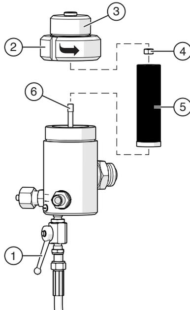
Fig. 25 Remove filter element
