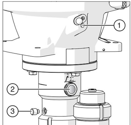
Fig. 24 Filling, checking, draining the release agent
