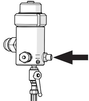
**Fig. 17** Connecting the spray hose to the high pressure filter
