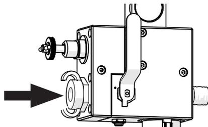
**Fig. 19** Connecting the compressed air (coupling is an example, not in scope of delivery)
