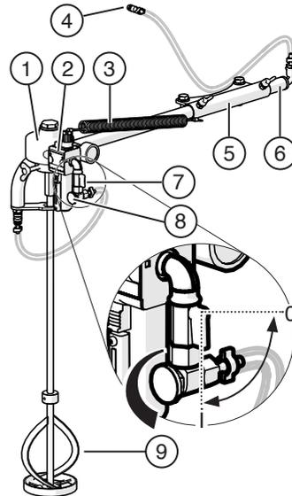
**Fig. 13** Pneumatic agitator as attachment kit
