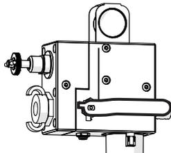
**Fig. 3** Compressed air shut-off valve OPEN
