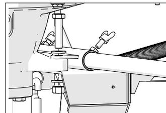
**Fig. 14** Screw on pipe mount and clamp agitator holder
