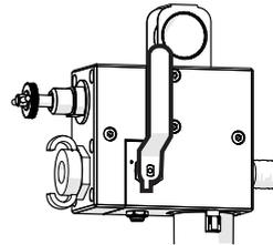
**Fig. 4** Compressed air shut-off valve CLOSED
