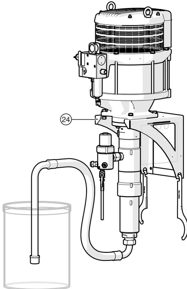
**Fig. 10** Herkules 333 GX on wall bracket
