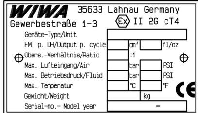
Fig. 28: Example of a type plate
