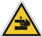
***To prevent serious harm by crushing or loss of limbs, do not work with the unit without the safety guards installed on all moving parts. Make sure that all of the safety protections are correctly reinstalled after all repair or maintenance work is completed.***
