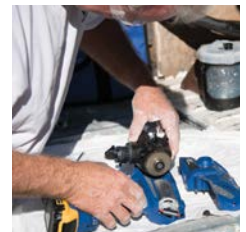
3. Place the new pump into sprayer.
