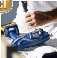
1. Remove the cover with a screwdriver.
