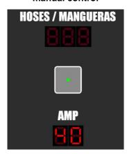
To select the temperature when the unit is working in automatic control mode, press the MODE key until the temperature flashes, select the required temperature by pressing the UP/DOWN keys and press the MODE key once more to enter the selected value into memory. Do the same process to select the Amps. When the unit is working in automatic mode, the value of the power must be set between 45 and 50 Amps.
