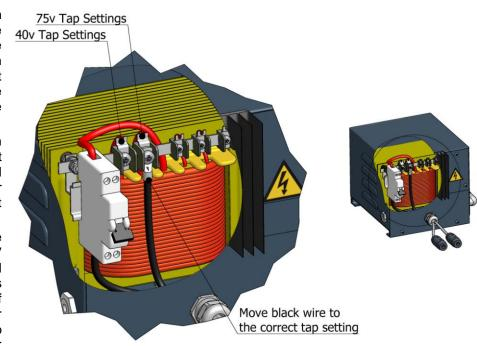
depending on the total hose length installed. Before starting up the unit, make sure that the connection made in the factory matches the total length of hose installed. If you add or eliminate sections of hose, make sure the output voltage of the transformer to which it is connected is suitable for the resulting total length. Otherwise, change the connection.
